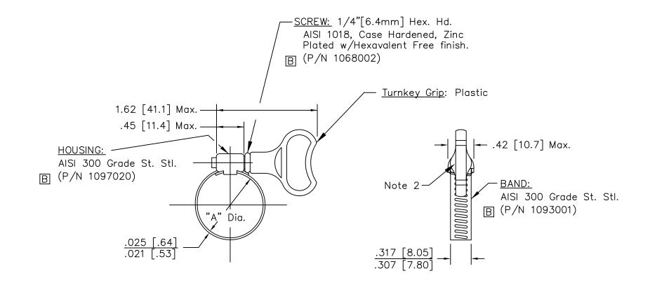
Torque Requirement: When mounted on a round steel arbor of "A" dia. max., less .062" [1.57mm], clamp must be capable of withstanding 20.0 in—lbs. [2.3 Nm] of torque applied by a hand torque wrench.
