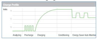
ChargePro's 5-Stage Performance Charging algorithm is fully automatic and designed to maximize battery performance and extend battery life.
